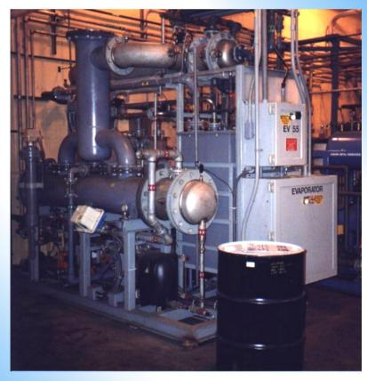
Vacuum evaporation system for the recovery of nitric acid, sulfuric acid and molybdenum. Produces 50-60 wt % nitric acid. Evaporator fabricated using 304L stainless steel with zirconium tube bundle, NEMA 4X electrical components, and PLC automation with PC interface.
